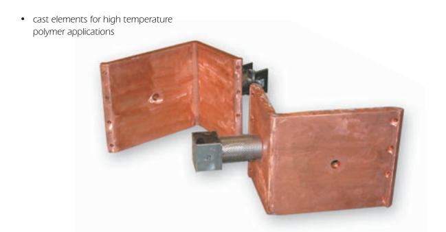
**Mounting:** Good thermal contact between the elements and metal surface to be heated is essential. Due to the large surface area and flat construction, warping of elements will result in air gaps, causing hot spots and possible failure of the element. It is therefore important that elements are clamped on tightly and that clamps are tightened again when the element has reached operating temperature.
