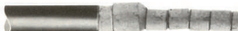
Ceramic beads over stranded NFg wire - length as required. 400°C Max Note: Limited bending radius
