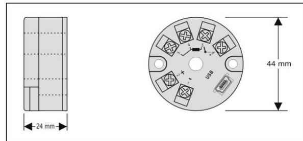
Fig. 4 – Transmitter dimensions
